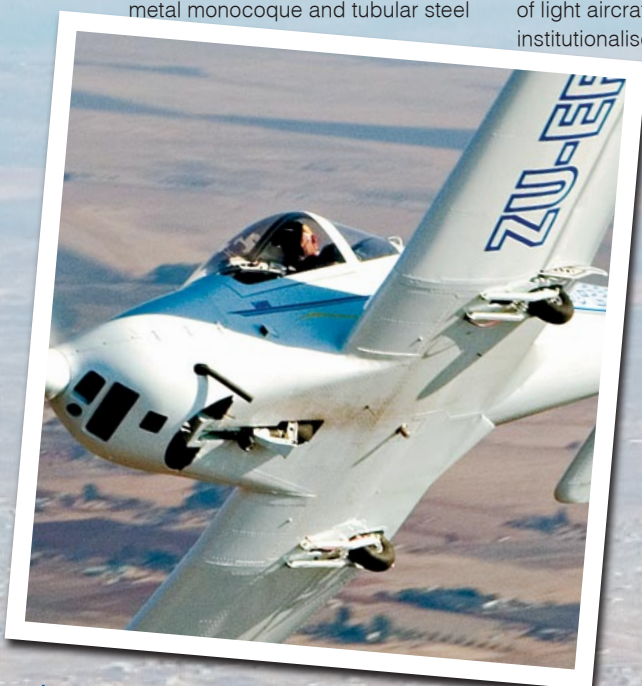
Left: Gear retraction configuration is very similar to earlier Zlin 326 and 526 models... and Russia's Yak 52
